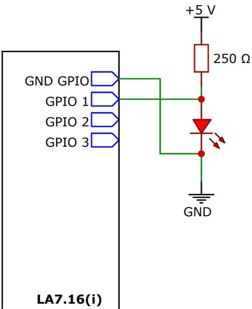
When the GPO is **closed**, the LED is **turned off** (the LED is short-circuited by the contact relay).
