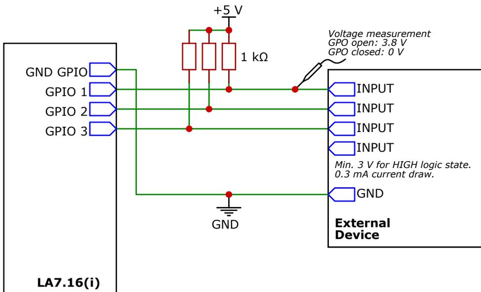
When the GPO is **closed**, the GPI of the external device is set to **LOW** logic state.
