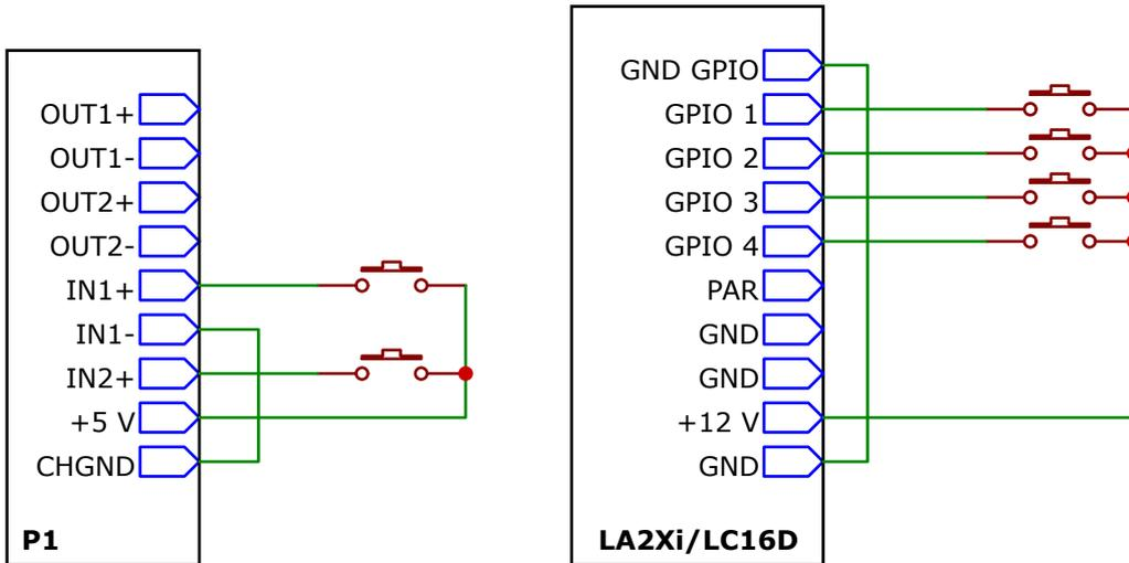
When the push button is closed, the GPI logic state is **HIGH**.
