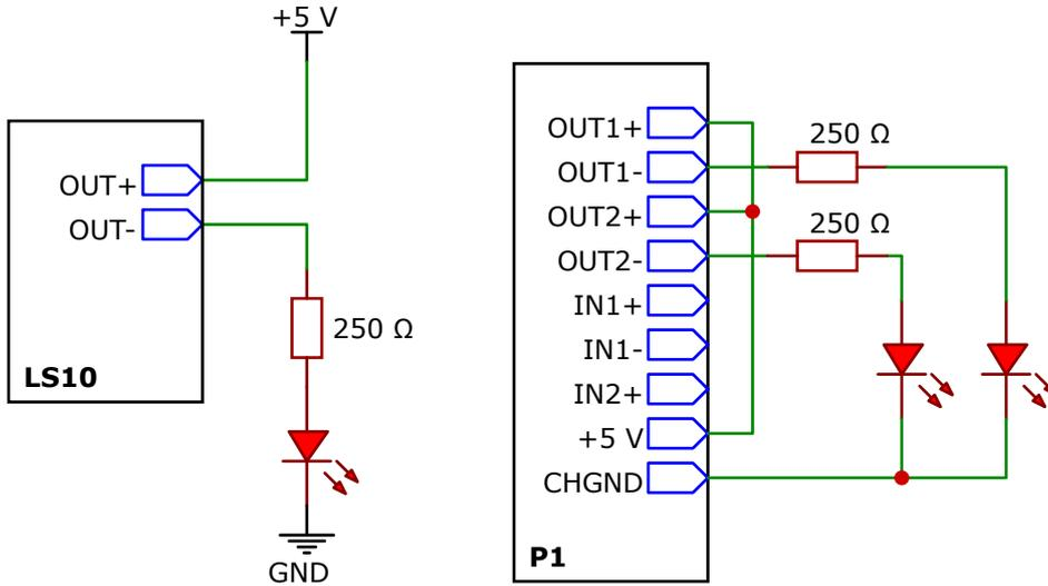
When the GPO is **closed**, the LED is **turned on**.
